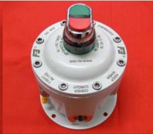
RJB11S2008 Key Switch and RJB11S2009, RJB11S2010 Selector Switches. Available in a variety of configurations: 0-1, 1-2, 1-0-2, 1-2-3, AUTO-MAN, FWD-OFF-REV etc. Up to 2 separate contacts available in each position. Choice of silver 690Vac or gold quad-connect low voltage contacts.
