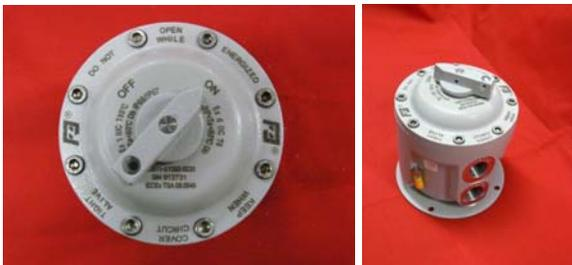
RJB11S1500 isolator and selector switches up to 4p 32A 11kW AC3. Feature padlockable handle, cable entries in the bottom side or top-bottom. Mounting base with 4 fixing points. External equipotential bonding connection facility for 4-6 mm<sup>2</sup> wire.
