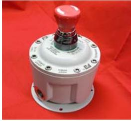
RJB11S2001 Emergency Stop. The robust external operator can be removed only with a special tool and can withstand shocks, impacts and vibrations as required by IEC60947-5-5. Latching operator, twist-to-release. Key release, locking and guard options available.
